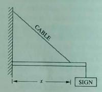
Design an algorithm to find the appropriate place (indicated by x in the diagram) to attach the cable to the pole so that the tension in the cable will be minimized. The equation governing static equilibrium tells us that
