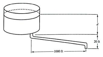
Several formulas have been developed experimentally to determine the velocity at which fluids flow through such pipes. One of these, the Manning formula, is
