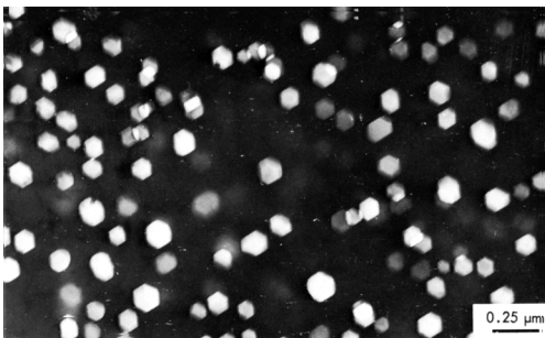
FIGURE 14 Void structure in irradiated stainless steel. [From M. T. Simnad and J. P. Howe (1979). In "Materials Science in Energy Technology" (G. G. Libowitz and M. S. Whittingham, eds.), Academic Press, New York.]
