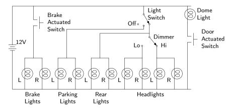
The designer of such a network needs to answer questions like: How much electricity flows when both the hi-beam headlights and the brake lights are on? We will use linear systems to analyze simple electrical networks.
